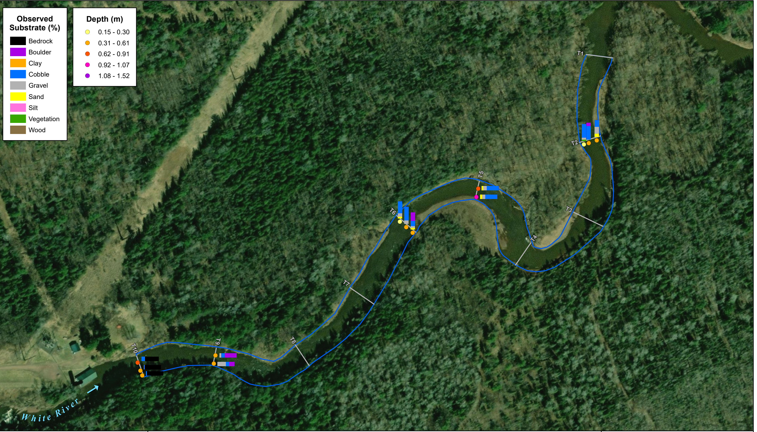
Figure 3. Substrate and Depth for the White River Project Reach Two on the White River. Ashland and Bayfield Counties, Wisconsin.
